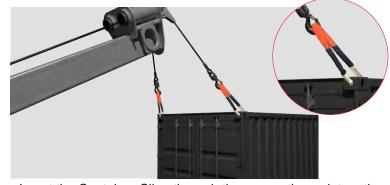
Insert the Container Sling through the connection point on the container. Ensure equal parts of the white *Dyneema* pad are on either side of the connection point.
