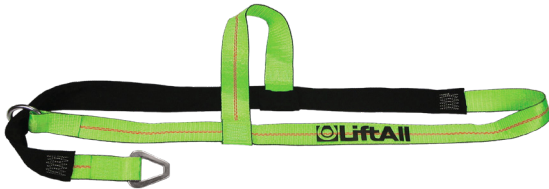
Basket Strap Wear Pad & Triangle End WLL 3,300-lbs. BSTRT
