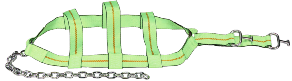
Cage Strap 2" Web • T-Hooks, 1/4"X26" G30 Chain WLL 1,600-lbs. **Used on Chevron ® and Challenger ® wheel lifts**
